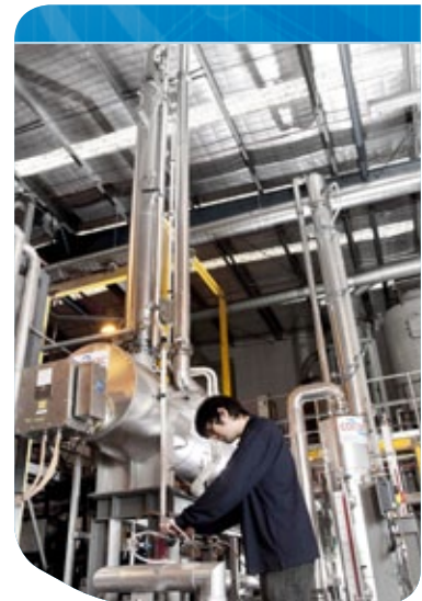
This solvent capture rig is being reconfigured for UNO Mk3 trials
