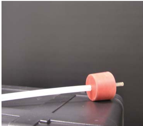
Figure 3. stopper and tubes assembled ready to install into the flask
