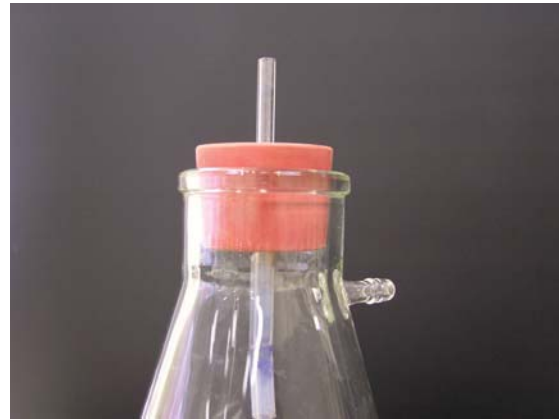
Figure 4. example of stopper and tubes installed in flask
